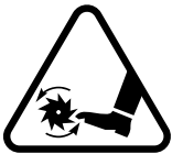
CUTTING HAZARD: KEEP FEET AND HANDS AWAY FROM ROTATING TINES.
